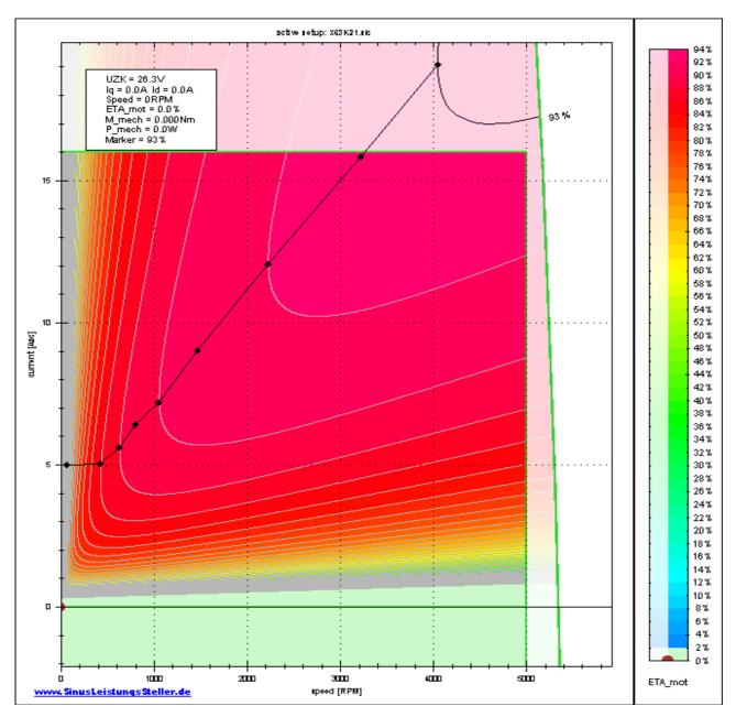
Lets watch the following ETA-plot of a typical BLDC-motor ...
