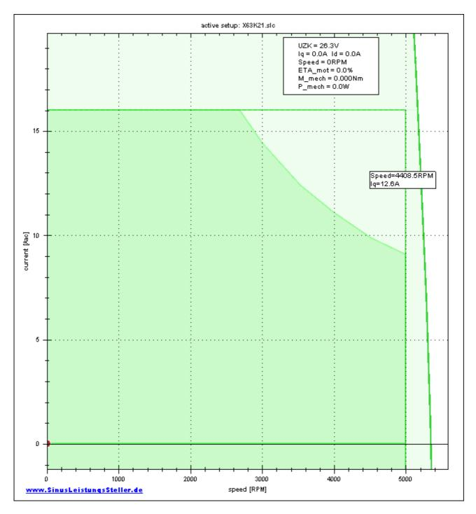
After saving the new \*.SLP-file and replacing it on SLS/SLR, the new limits (incl. max. 250W P\_mech) in "OperationPointLive" now looks like:
