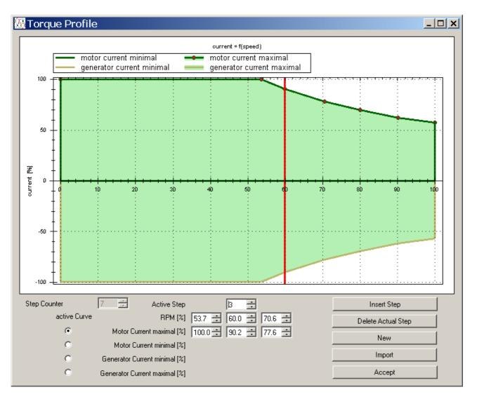
If Option TorqueProfile was not enabled the SLS/SLR-device, the edit function is not available - values can't be modified but watched.
