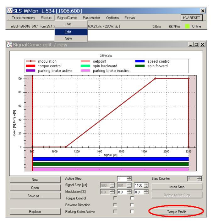
If no TorqueProfile attachment was found and no TorqueProfile-option is enabled, the "TorqueProfile "-button will stay inactive (grayed).
