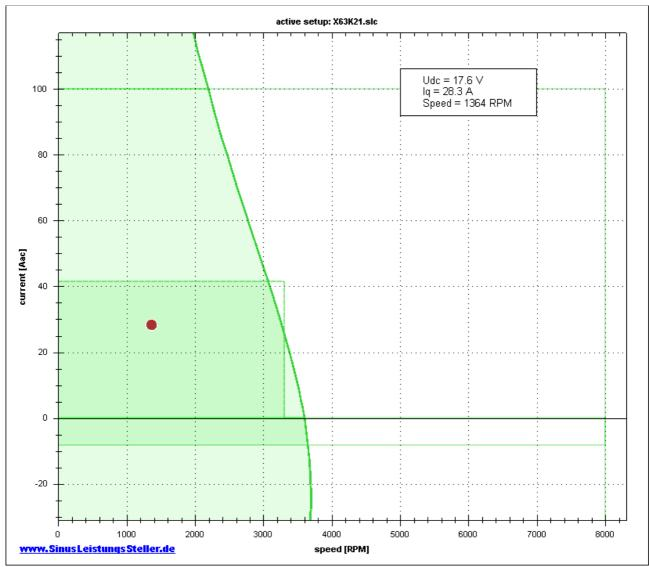
$(Udc_low_lim = 18.0V \rightarrow derating is active in picture above, limits are folded back)$
