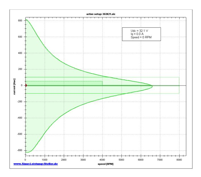
Working points on the enveloping curve marks the theoretical limit of phase-current vs. speed. The drop in speed vs. load can be readout directly from this diagram following the green line.
