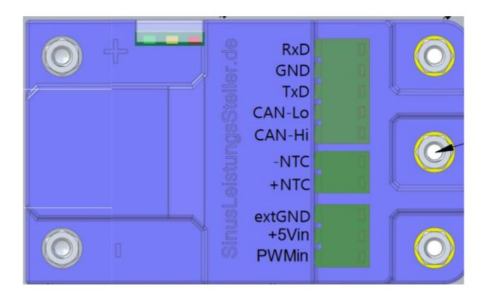
The +5Vin have to be supplied to the mSLR from the outside, because the internal optocoupler needs also to be supplied.
